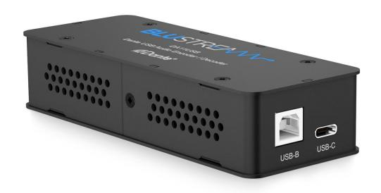
Our DA11USB has been designed to both encode a 1ch mono (L/R channels merged) USB audio input to a Dante® output digital signal, and also decode a Dante digital input signal back to 2ch USB output audio.
