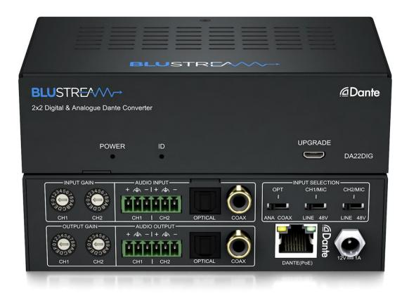
Our DA22DIG has been designed to encode 2ch analogue or digital audio inputs into a Dante® digital signal, and decode 2ch Dante digital signals to the simultaneous analogue and digital audio outputs.
