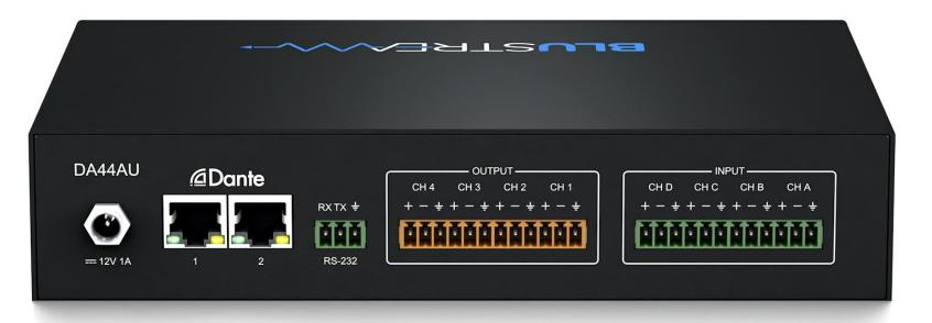
Our DA44AU is a 4 x input, 4 x output Dante® audio converter. The DA44AU allows any non-Dante audio source such as mixing consoles, amplifiers, computers and Blustream Matrix / distribution products to be connected as analogue audio sources to a Dante network, as well as converting up to 4 x mono / 2 x stereo Dante signals back to analogue audio.
